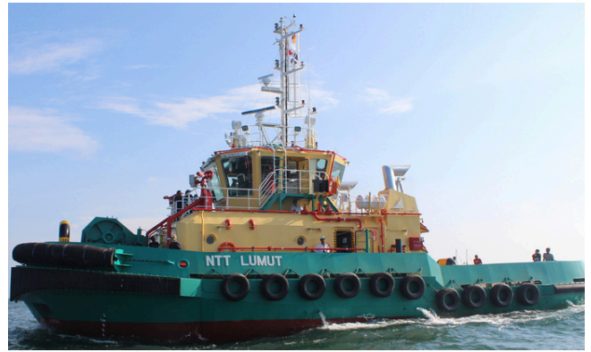
NTT-LARUT, LUMUT, Daihatsu Propulsion Engine 6DKM-26e(F)(L) with Kawasaki Rexpeller and Jason FiFi
