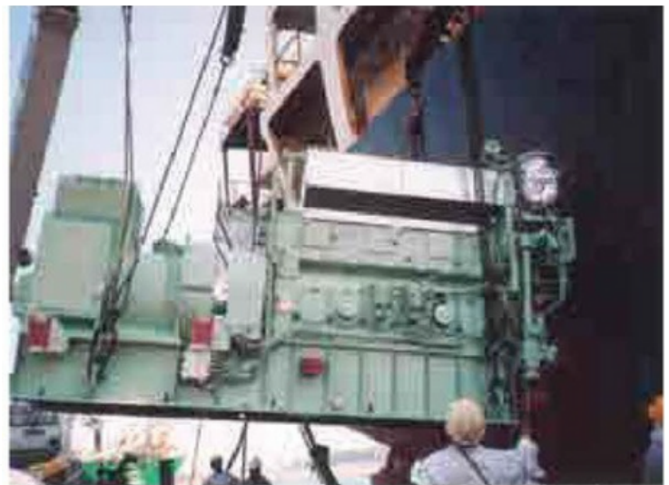
Installation of Daihatsu Engine 6DK-20 onboard the vessel Shaktidoot
