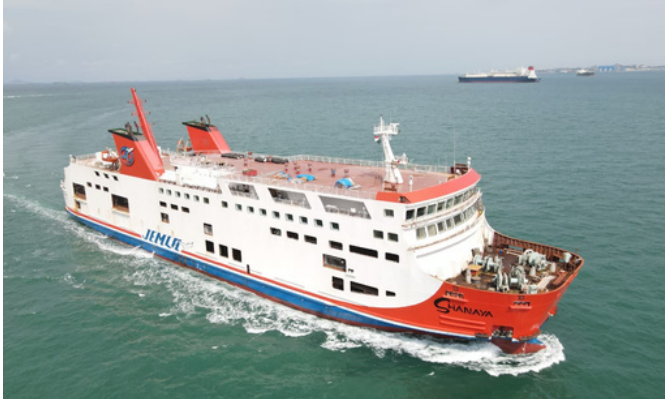
KMP SHANAYA 120m RoRo Passenger Ferry, Daihatsu Propulsion Engine 6DKM-36e(L) and Daihatsu Generator 6DE-18
