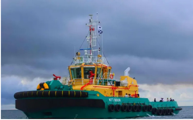
NTT-BATIK, BERCHAM, BERUAS, BIDOR, Daihatsu Propulsion Engine 8DKM-28eF(L) with Kawasaki Rexpeller and Jason FiFi
